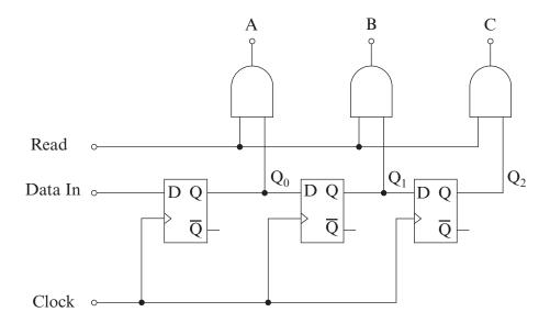
Complete the graphs opposite to show the outputs  $Q_0$ - $Q_2$ , and A-C in response to the given 'Clock', 'Data In' and 'Read' signals.
