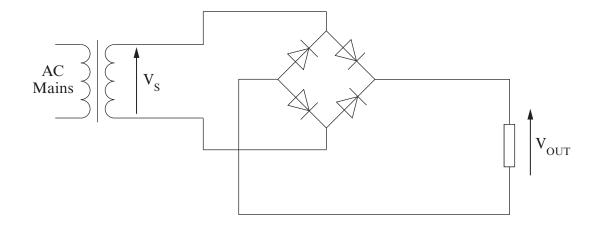
(a) The **peak** value of the secondary voltage of the transformer ( $V_S$ ) is 6 V. Calculate the **peak** value of the full-wave-rectified voltage  $V_{OUT}$ .
