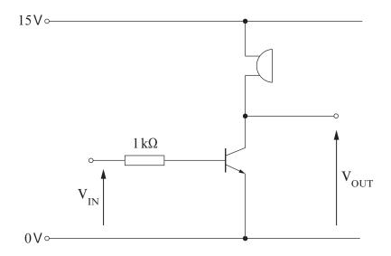
(a) The transistor has a current gain,  $h_{FE} = 75$ .
