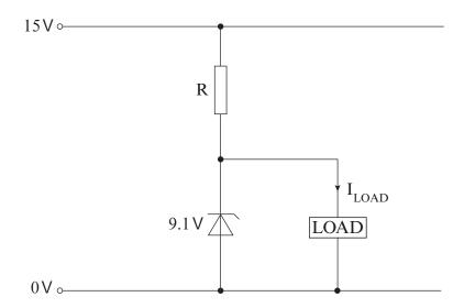
The power supply must be able to supply a load current,  $\boldsymbol{I}_{LOAD}$ , of  $300\,\text{mA}.$
