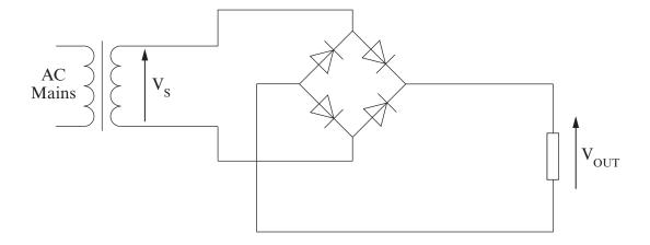
(ii) A large current is drawn from the smoothed full-wave-rectified power supply. Use the next set of axes to sketch the voltage  $V_{\rm OUT}$ .
