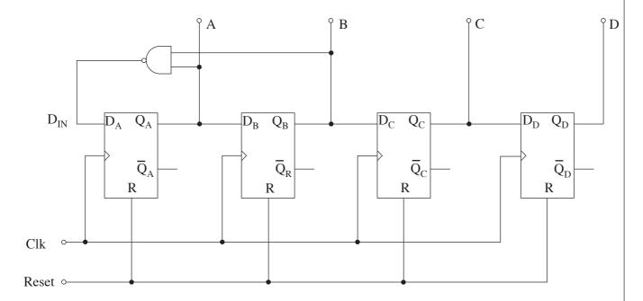
The shift register is reset so that outputs A, B, C, and D are logic 0. Complete the following table to give the state of the output after the given number of clock pulses have been applied. [4]
