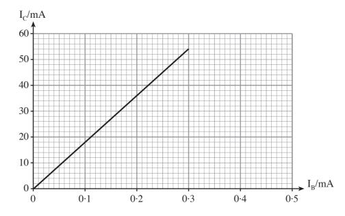
Determine the current gain  $(h_{\text{FE}})$  of the transistor.
