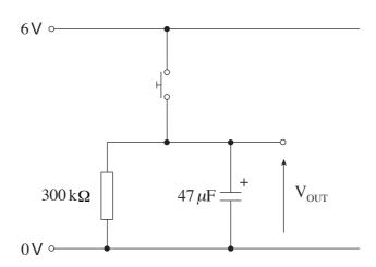
(a) Calculate the time constant of the timing system.
