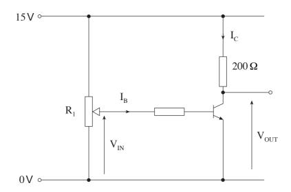
Potentiometer  $R_{\rm l}$  is varied and readings of  $V_{\rm IN},\,V_{\rm OUT},\,I_{\rm B}$  and  $I_{\rm C}$  are taken.
