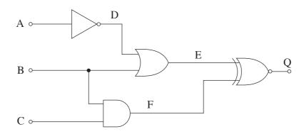
(a) Give the Boolean expressions for the outputs D, E and F of the gates in the logic system in terms of A, B and C. [2]
