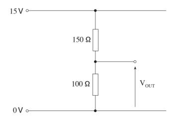
(a) Thevenin's theorem is used to produce an equivalent circuit.
