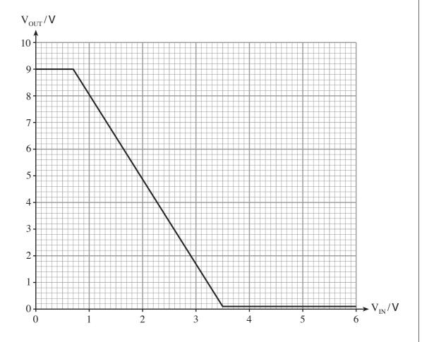
Use the graph to determine the minimum value of  $\boldsymbol{V}_{\text{IN}}$  required to saturate the transistor
