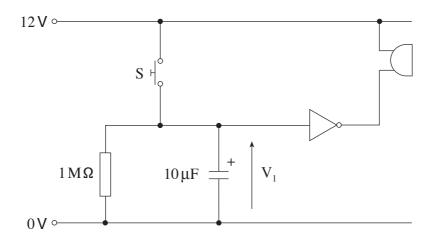
The CMOS inverting buffer (NOT gate) has the following parameters when connected to a  $12\,\mathrm{V}$  power supply:
