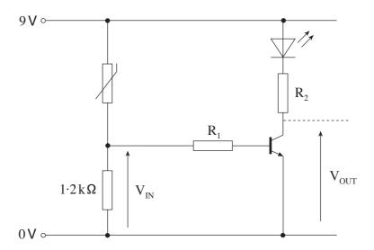
(a) The temperature is gradually increased. The graph shows how  $V_{\rm IN}$  and  $V_{\rm OUT}$  change.
