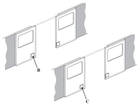
Switch A [not shown] is a motion sensor that outputs logic 1 when the train begins to move. When a door is open, its sensor, **B** or **C**, outputs logic 0. The output **Q** of the electronic system becomes logic 1 and triggers the alarm if either or both doors are open as the train begins to move.
