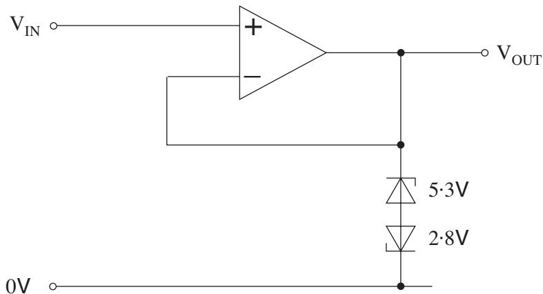
Draw the switching characteristic of the Schmitt trigger when the op-amp is connected to a  $\pm 12V$  power supply using the axes below.
