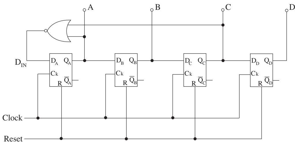
The shift register is momentarily reset so that outputs A, B, C and D are logic 0. Complete the following table to give the state of the output after the given number of clock pulses have been applied. [4]
