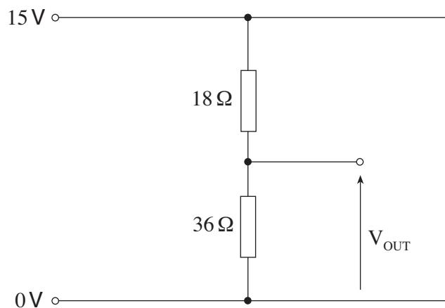
(a) Thevenin's theorem is used to produce an equivalent circuit.
