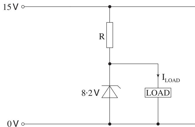
The power supply **must** be able to supply a load current,  $I_{LOAD}$ , of 60 mA.
