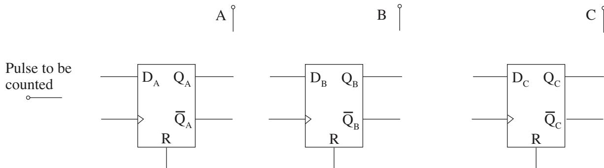
(ii) On the circuit diagram above add a logic gate and the connections necessary to make the counter reset on the fifth clock pulse. [3]
