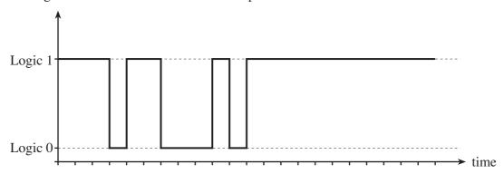
(a) The signal includes a start bit and two stop bits, a parity bit, and 7 data bits corresponding to the ASCII character.
