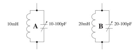
Which circuit, A or B, provides the user of the radio with the ability to select a frequency range between 120 kHz and 250 kHz. You must show all of the calculations you have performed.
