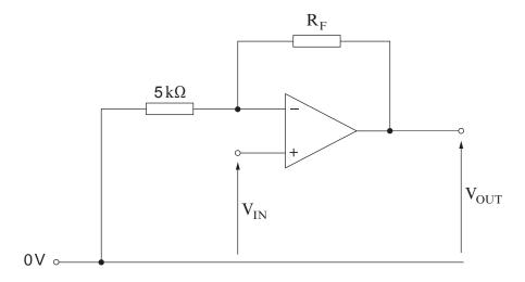
(a) (i) Calculate the value for resistor  $R_{\rm F}$  such that the voltage gain of the amplifier is 9. [1]
