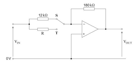
The op-amp is powered from a  $\pm$  15 V supply and saturation occurs at  $\pm$  14 V. An input voltage of 0.9 V is applied to  $V_{\rm IN}.$
