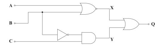
(a) Give the Boolean expression for each of the outputs X, Y and Q in terms of the inputs A, B and C.
