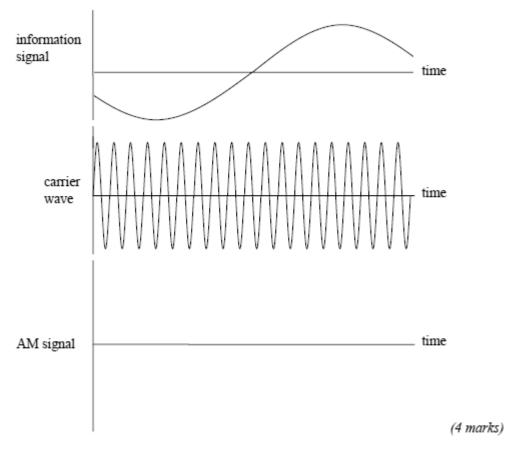
3 (b) The information signal has a maximum frequency of 4.5 kHz and the modulated carrier is to be transmitted on the MW band.
