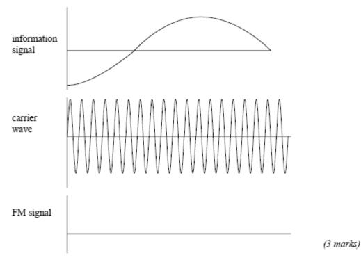
3 (b) The information signal has a maximum frequency of 15 kHz, the maximum frequency deviation of the carrier is ± 75 kHz.
