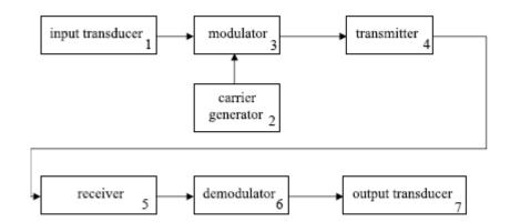
(a) Describe the type of signal that passes between each pair of numbered subsystems.
