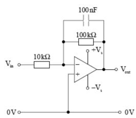
Calculate the reactance of the 100 nF capacitor at a frequency of 20 Hz.
