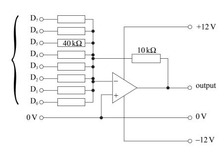
(i) Calculate the values for the resistors for the  $D_6$  and  $D_1$  inputs.
