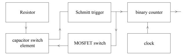
The capacitor switch element charges through the resistor.
