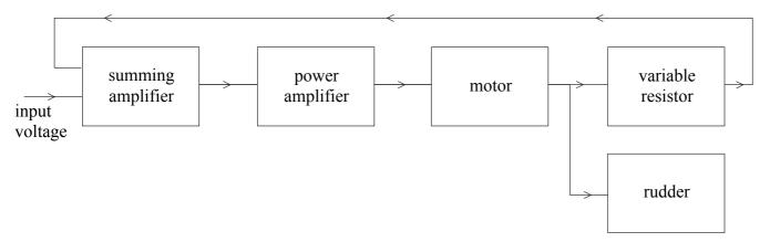
As the motor rotates it alters the position of the rudder and the variable resistor. The variable resistor sends a control voltage back to the summing amplifier.
