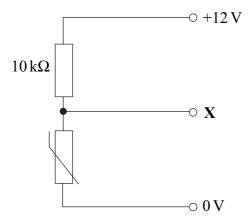
(a) The thermistor shown above has a resistance of  $30\,\mathrm{k}\Omega$  at  $0\,^\circ\mathrm{C}$ ,  $15\,\mathrm{k}\Omega$  at  $25\,^\circ\mathrm{C}$ , and  $2\,\mathrm{k}\Omega$  at  $100\,^\circ\mathrm{C}$ .
