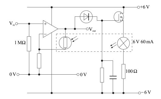
The lamp and LDR are in a sealed container so that only light from the lamp illuminates the LDR.
