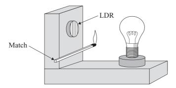
When a lighted match is held near to the LDR, the lamp lights and remains lit even when the match is removed.
