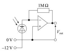
The photodiode current in the dark is  $0.1 \,\mu\text{A}$  and in the light is  $6 \,\mu\text{A}$ .
