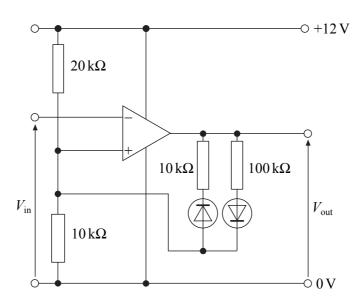
Assume that the op-amp is ideal and the diodes have no forward voltage drop and zero reverse leakage current.
