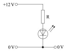
Calculate a suitable preferred value for the resistor, R.
