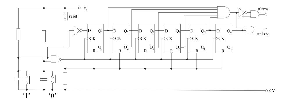
To operate the lock, the circuit is first reset and then a binary number is entered by pressing the '1' and '0' switches. If an incorrect number is entered an alarm is sounded.
