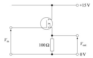
(a) An alternating voltage of 10 V amplitude is supplied to the input of the source follower as shown in the graph below.
