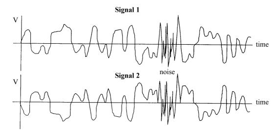
**Signal 1** is connected to input A of a summing amplifier. **Signal 2** is passed through an amplifier with a voltage gain of -1 and then connected to input B of the summing amplifier, as shown in the diagram below.
