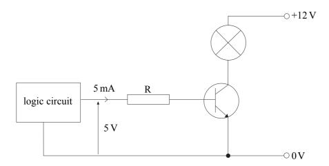
(a) The base-emitter voltage of the transistor when switched on is 0.7 V.
