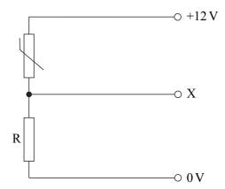
(a) The thermistor used in the circuit has a resistance of  $45\,k\Omega$  at  $0\,^{\circ}C$ ,  $13\,k\Omega$  at  $25\,^{\circ}C$  and  $1\,k\Omega$  at  $100\,^{\circ}C$ .
