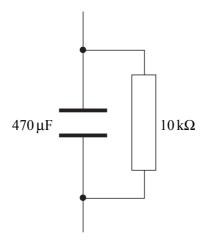
(a) Calculate the time constant of the circuit.
