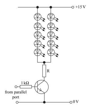
(ii) State the maximum current that has to be switched by the transistor.
