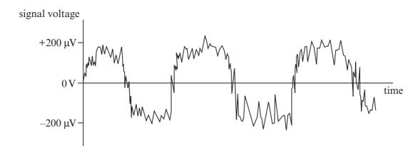
(a) This signal is amplified by an inverting amplifier with an input resistance of  $10 \, \mathrm{k}\Omega$  and a voltage gain of -200. In the space below, draw the circuit diagram of such an op-amp based amplifier. Mark on your diagram suitable values for the resistors.
