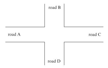
The microcomputer system is programmed to minimise the waiting time for vehicles. To detect how many cars are waiting on each road, a wire sensor is laid into the surface of each road which alters the frequency of an astable oscillator. The more vehicles that are waiting, the lower the frequency.
