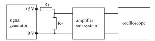
The signal generator is set to 5 V and connected to two resistors arranged as a voltage divider. If  $R_1$  = 1 M $\Omega$ , calculate the value of  $R_2$  so that the input signal to the amplifier is 5  $\mu$ V.
