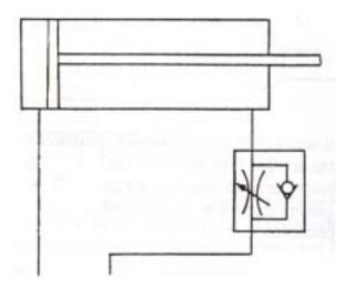
(c) System used must ensure cylinder F is in-stroked or instroking. Shown is time delayed outstroke of an SAC. Air for new part of circuit derived from mains air to instroke cylinder F. As below or similar. Up to [2] for good explanation. Up to [2] for working circuit.
