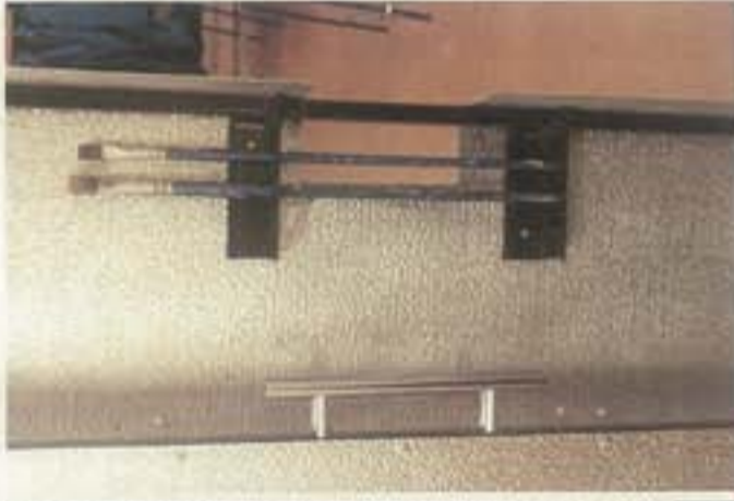
Left door with 2 brushes in the holder. Note that 3 brushes can be held at any one time.
