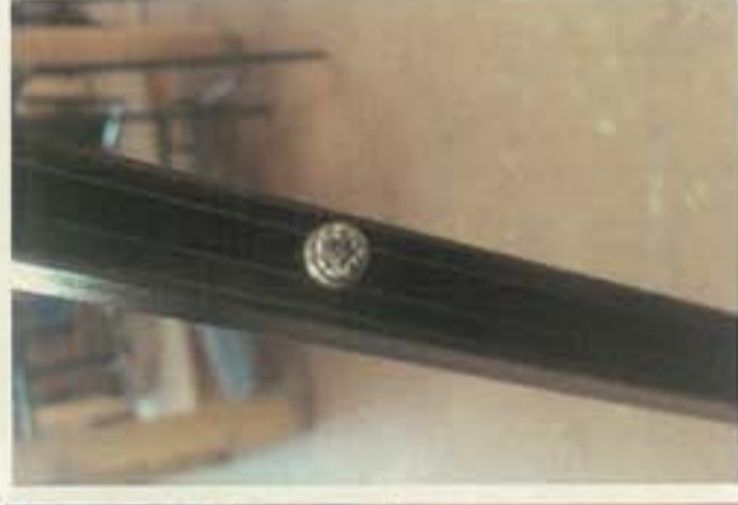
Slotting mechanism of the back leg. It is used to adjust the overall height.
