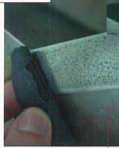
Before filing, the desired curve is marked out on the aluminium using callipers. Firstly, aluminium is removed using a dreadnought file, pictured below. Once a lot of material is removed, a normal file is used to clean up the edges and get it into the desired shape.
