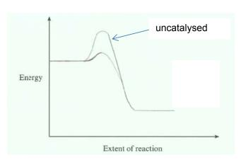
exothermic profile drawn (1) uncatalysed / catalysed line labelled (1) [2]
