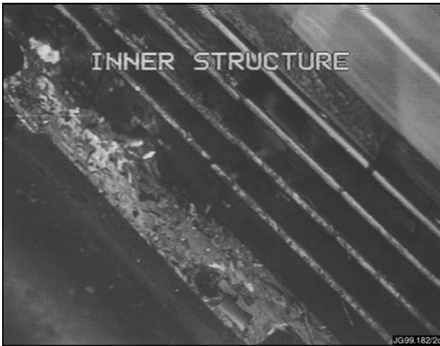
Fig. 4 Photograph of flakes and dust resulting from the break-up of hydrocarbon films deposited on cool surfaces in the tokamak
