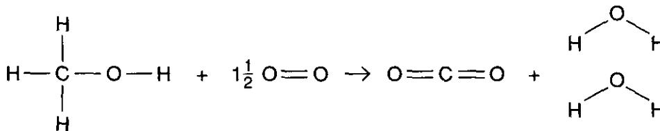
Use the average bond enthalpies from Table 2.1 to calculate the enthalpy change of combustion of gaseous methanol,  $\Delta H_c$ .
