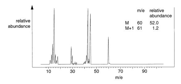
Use the M and (M+1) peaks in the mass spectrum to determine the number of carbon atoms present in  $\mathbf{P}$ .
