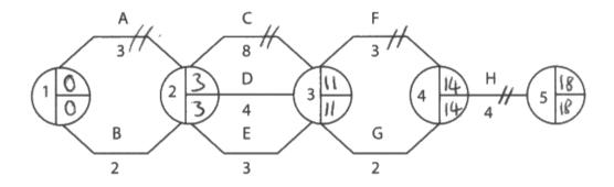
(a) Using the data in the network diagram above, calculate the Earliest Start Times (EST) and Latest Finishing Times (LFT) for each activity and identify the critical path.
