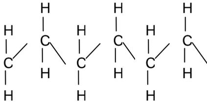
High Density Polyethylene (HDPE) has long chains like in the diagram above. It is made using complex catalysts at low temperatures (350 K). Because it has few side chains the chains pack together closely and it has 75 – 95% crystallinity. It therefore has greater strength and stiffness than Low density Polyethylene (LDPE) which is made using simple catalysts at higher temperatures and has only 55 -70 % crystallinity.
