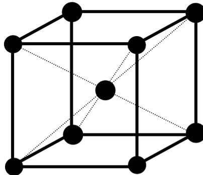
Pure iron has little practical value. Add carbon to make the alloy steel. The extra carbon atom is an interstitial (extra atom between existing ones).
