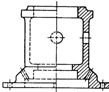
Why is a half-section view sometimes used in the preparation of orthogonal drawings?
